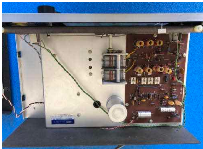
Figure 5: Top interior view of the SW-717. Note the circuit board to the right and the main tuning capacitor and can capacitor along the center. The twisted blk/whi wires go to the speaker attached on the cover partially visible to the left
